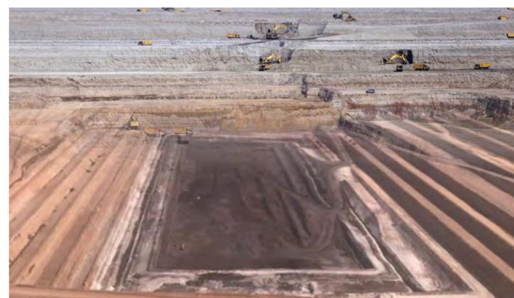
strips to enable excavation of the coal seams. This is done through using large machines, removing strips of overlying soil and rock and then excavating coal deposits;
