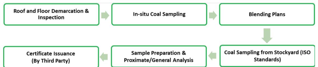
Fig. 03: Flow chart showing the coal blending, sampling and testing regime
